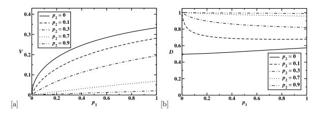
Figure 5: Dynamic properties of the unbiased molecular motor with u = w = 1 and with the concentration of bridges c = 0.2: (a) The mean velocity as a function of the burning probability for different recovery probabilities; (b) dispersion as a function of the burning probability for different recovery probabilities.
