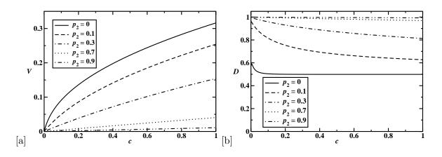
Figure 3: Dynamic properties of the unbiased molecular motor with u = w = 1 and with the probability of burning  $p_1 = 0.1$ : (a) The mean velocity as a function of the concentration of bridges for different recovery probabilities; (b) the dispersion as a function of the concentration of bridges for different recovery probabilities.
