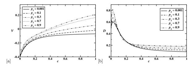
Figure 7: Dynamic properties of the backward biased molecular motor with u = 0.3 and w = 0.7, and with the recovery probability  $p_2 = 0.1$ : (a) The mean velocity as a function of the concentration of bridges for different burning probabilities; (b) the dispersion as a function of the concentration of bridges for different burning probabilities.
